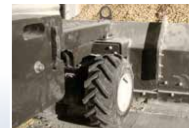
Tires Are Foam Filled, With Tractor Tread.
